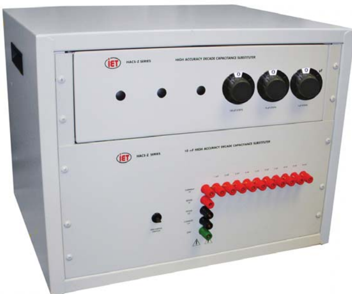
HACS-Z High-Capacitance Substituter: 4-decade, 1 \mu\text{F} through 1000 \mu\text{F} steps
